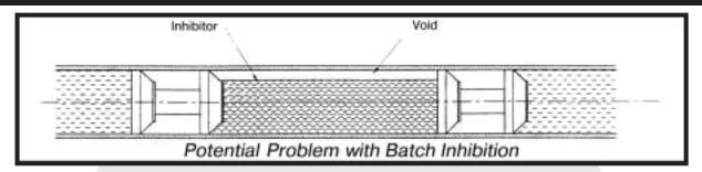
For batch separation or meter proving, the sphere may be pressurized to size it just slightly larger than the pipe inside diameter to give a good seal. When pigging for condensate removal however, it is common to size the sphere to equal the pipe inside diameter which will allow the sphere to roll and minimize the wear.
