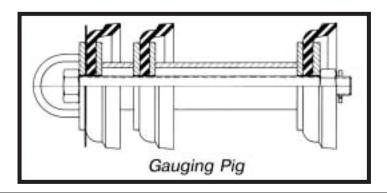
the flange would push any construction debris out of the pipeline, or the pig would stop if it encountered an obstruction.
